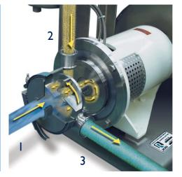
Inline SLIM. The liquid stream (1) enters the mixer and immediately encounters the powder injection (2) at the high shear zone of the rotor/stator assembly. The resulting dispersion (3) is expelled centrifugally through the stator openings at high velocity.
