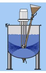
**Batch SLIM.** As the rotor reaches operating speed, the SLIM valve is opened and powders are quickly drawn into the batch by virtue of the powerful vacuum generated by the ported rotor.
