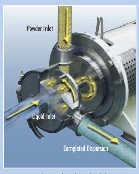
An intense vacuum draws powders including silica, thickeners and pigments into the mix chamber of the SLIM Solids/Liquid Injection Manifold. They are injected through a ported rotor directly into the high shear zone and dispersed instantly.
