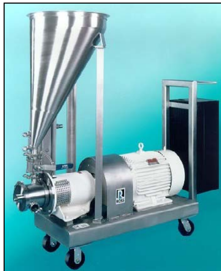
Fig. 2: Ross Model ME-405SB/25 with hopper arrangement All factors being equal, the hopper is preferred as it:
